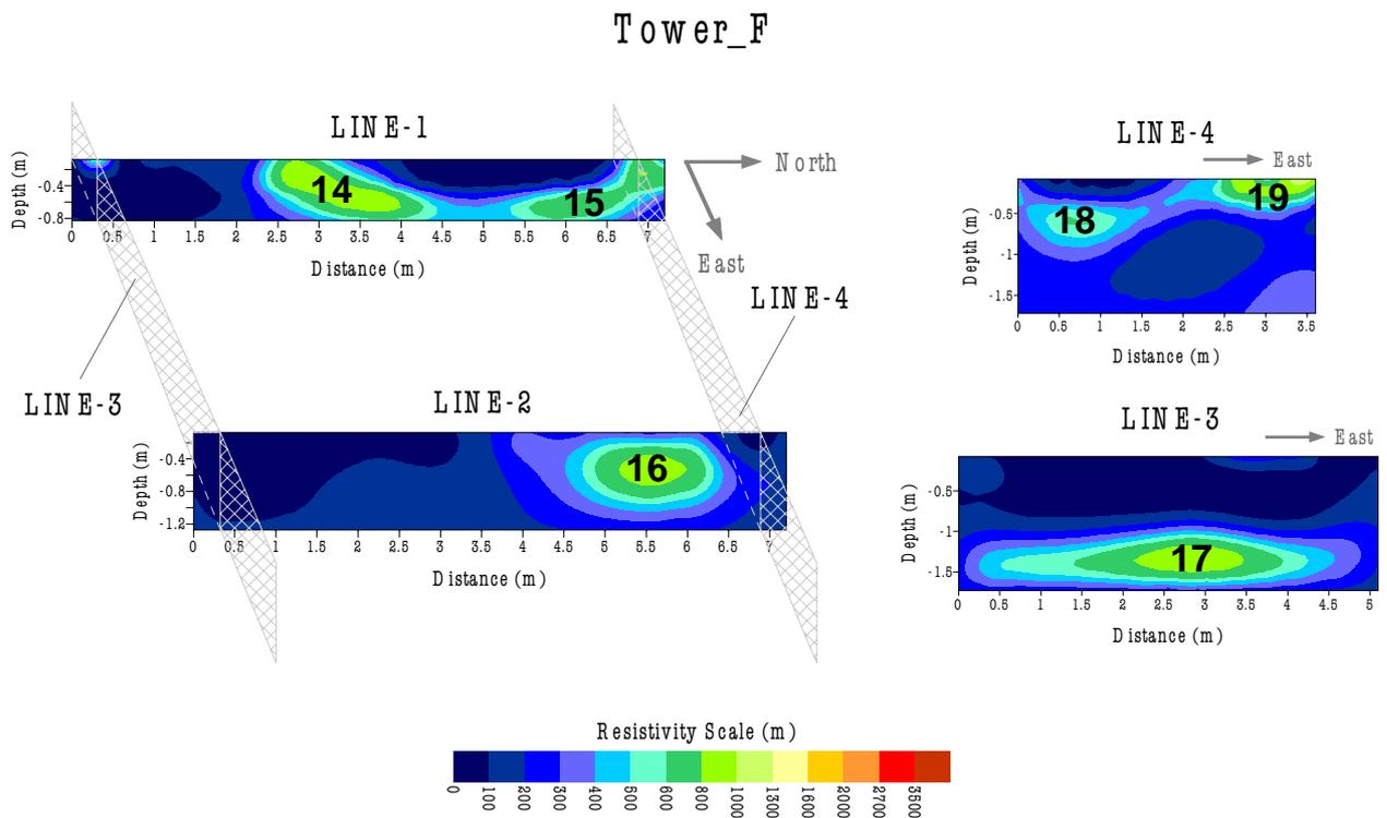
FIG. 14. 2D resistivity tomograms in the placement area of tower F.
