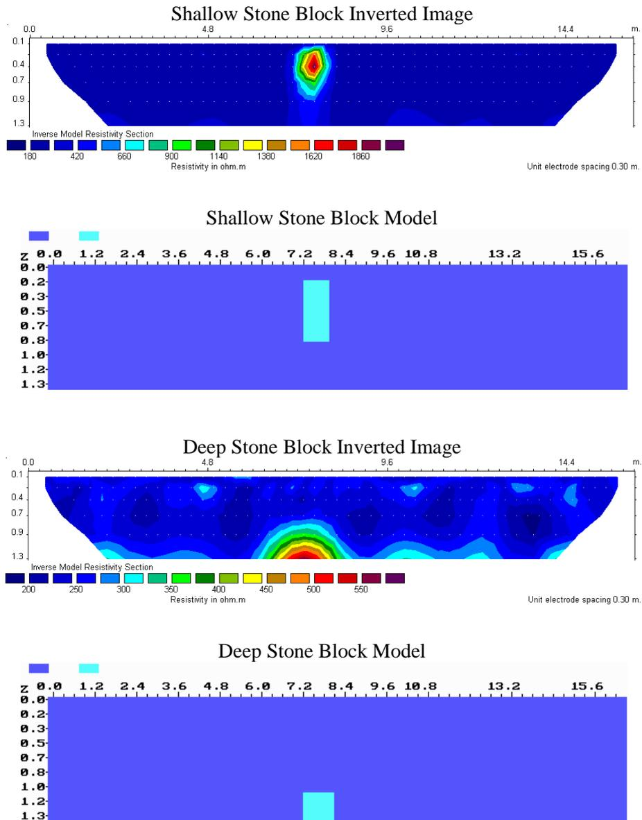
FIG. 6. Synthetic modelling results for the stone model.
