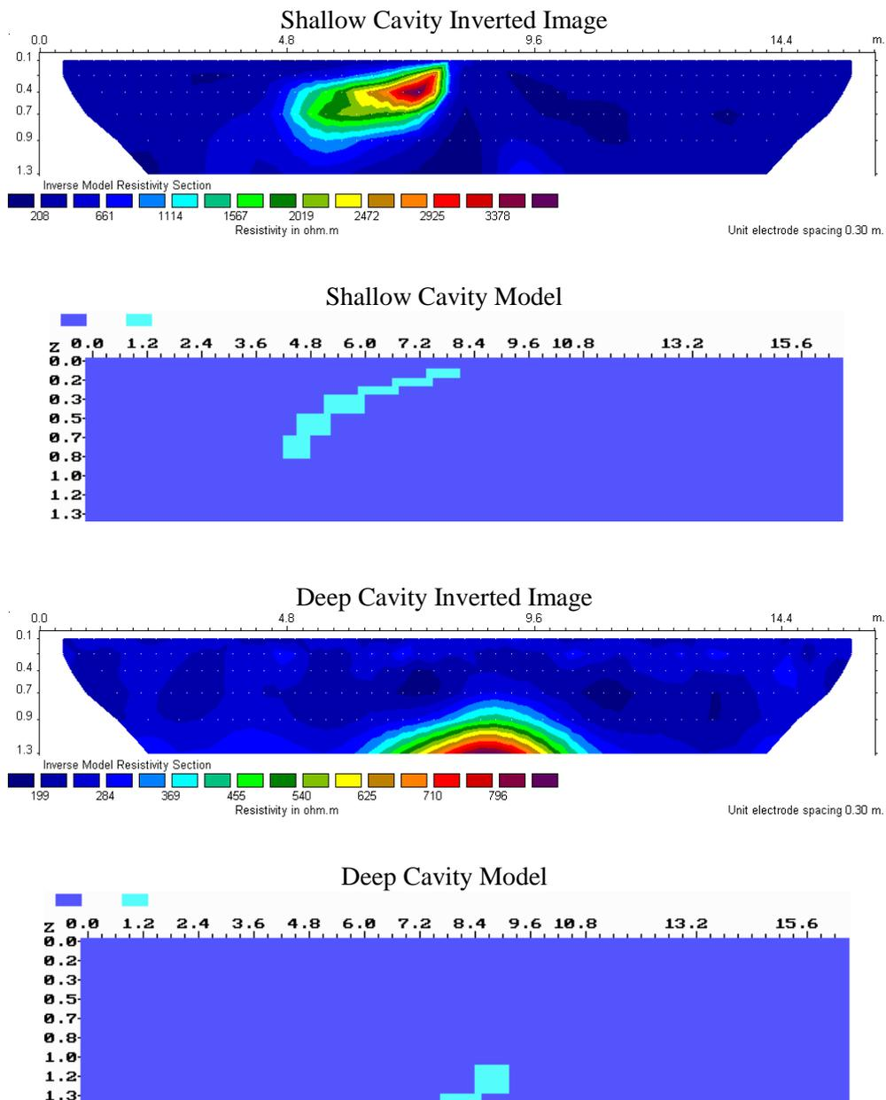
**FIG. 5.** Synthetic modelling results for the cavity model.
