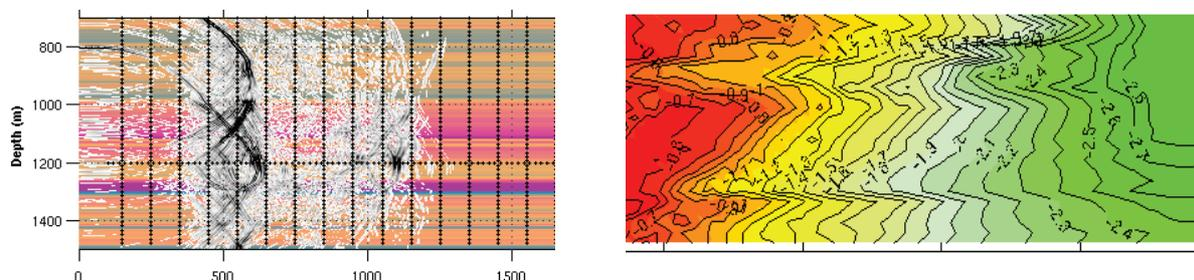
**Figure 1** a) (left) waveform modelling for the analysis of waveform complexity. b) (right) Network sensitivity for  $n$  array deployed mid-depth above the target based on the waveform analysis.
