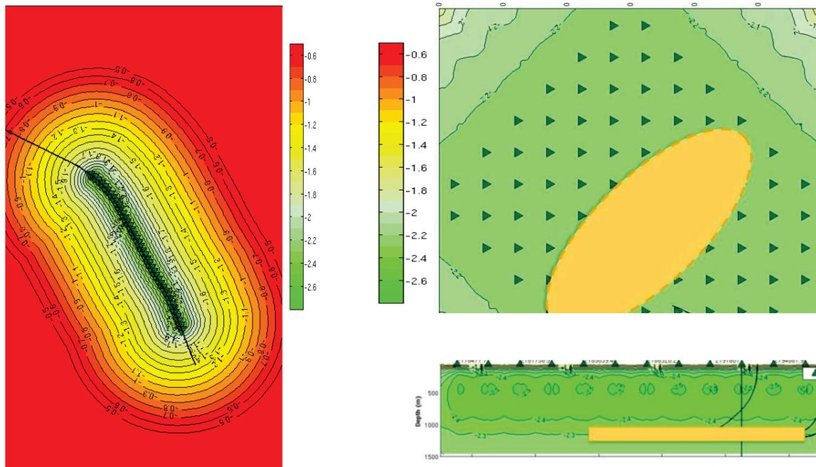
**Figure 2** Comparison of the distribution of minimum magnitude detectable with a borehole and a surface array. a) (left) horizontal cross-section through the target area including the horizontal monitoring well; low magnitude events can be detected in the vicinity of the observation well but the coverage is uneven. b) (right) same parameter mapped in a horizontal and in a vertical cross-section through the target zone: even coverage but decreased magnitude with depth.
