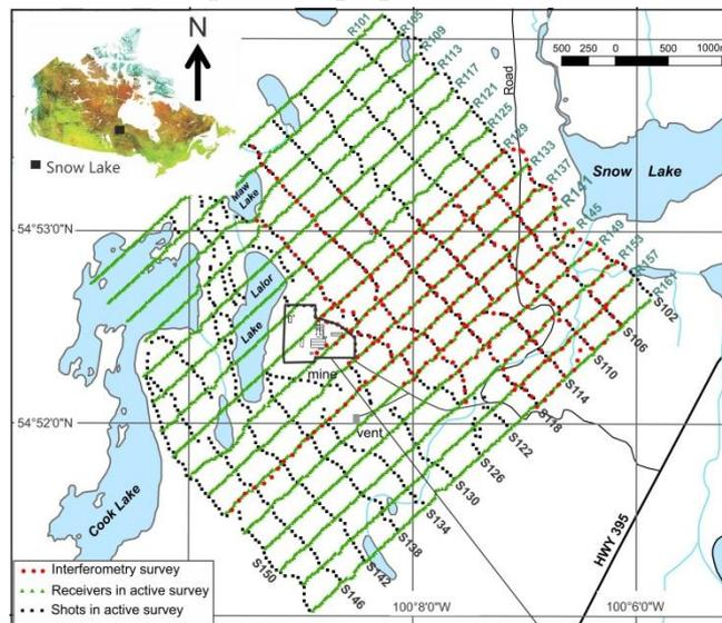
**Figure 1** Geometry of the active 3D survey and the interferometry survey in the Lalor mining area. The active and interferometry surveys cover approximately 16 km<sup>2</sup> and 4 km<sup>2</sup>, respectively. The mine area and ventilation shaft is also shown. The inset figure shows the location of Snow Lake, Manitoba.
