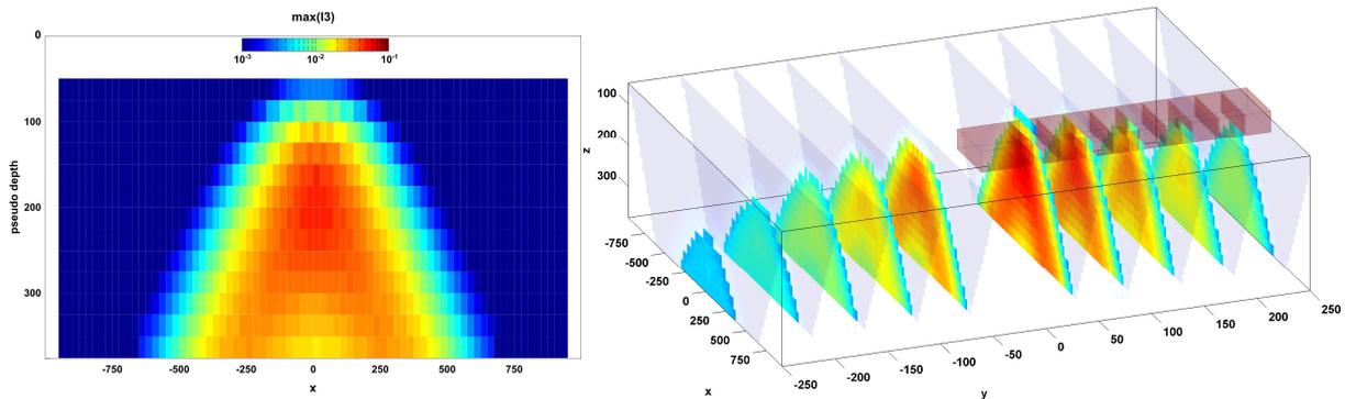
**Figure 2** Skew invariant (maximum of absolute value) for anomalous body (right, block structure), calculated for various TX-RX offsets and positions. For each TX-RX combination the according value is plotted at the midpoint between TX and RX at a pseudo depth of half the TX-RX offset (left: section at  $y = 25\text{m}$ ; right: anomalous body with collection of pseudo sections).
