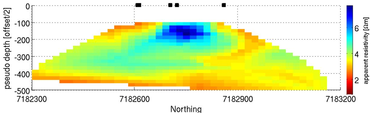
**Figure 3** Apparent resistivity section (interpolated) from measurements conducted on the Norwegian shelf, Nyegga area. Black squares mark the projection of five receivers onto the profile line.
