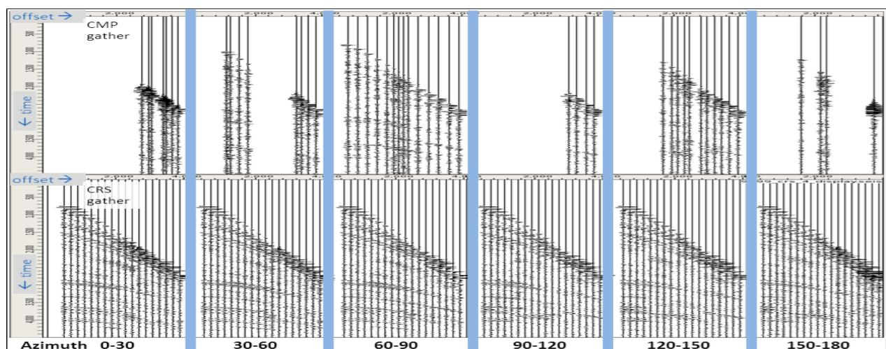
**Figure 1** Initial CMP gather (top) versus CRS gather (bottom) at the same CMP location with azimuth decomposition at intervals of 30 degrees.
