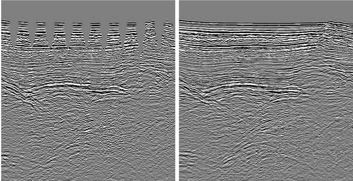
**Figure 2** Initial CMP stack (left) and CRS stack at the central azimuth of 105 degrees.
