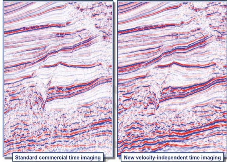
Figure 2 It can be seen the excellent detention of thrust faults, the greatly improved S/R and the overall improvement due to the best focusing.
