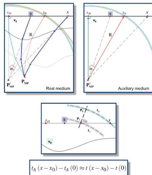
Figure 1 *Quasi-similar 2D Earth models and time delay: the image of  $P_{\text{NIP}}$  is determined in the auxiliary medium by the center  $P_{\text{NIP}}^*$  of the osculating circle tangent in  $x_0$  to the emerging diffraction wave.*
