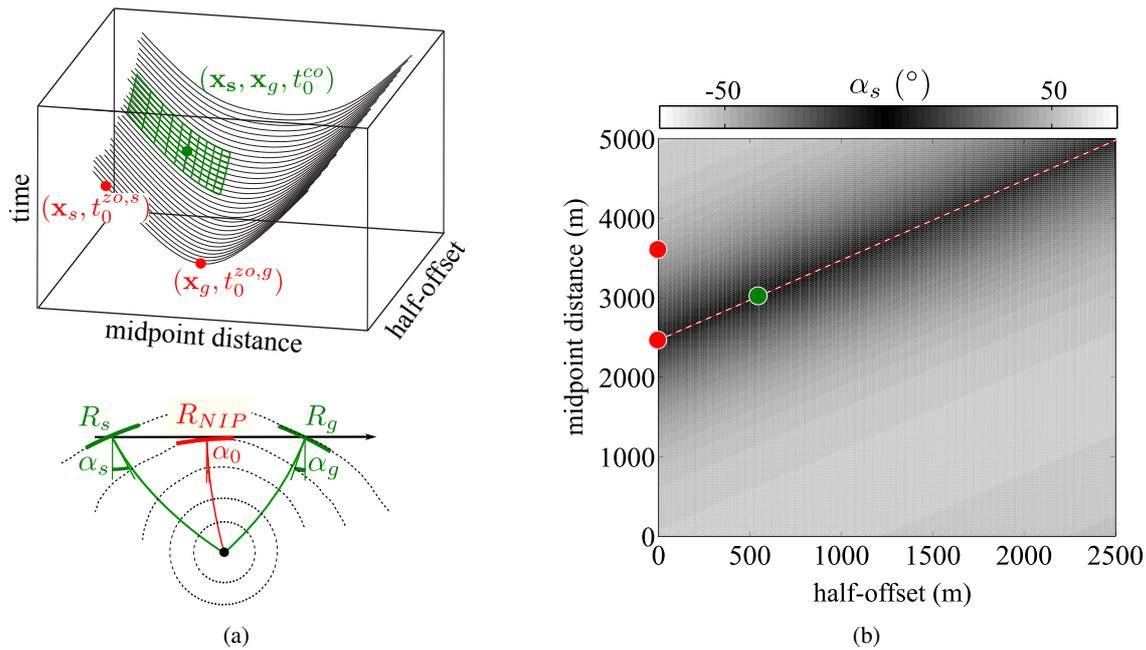
**Figure 1** (a) Illustration of the connection between ZO (red) and CO (green) information for the diffraction case. (b) CR wave emergence angle as a function of midpoint distance and half-offset. The coloured dots mark the ZO (red) and CO (green) locations that were considered in the synthetic test.
