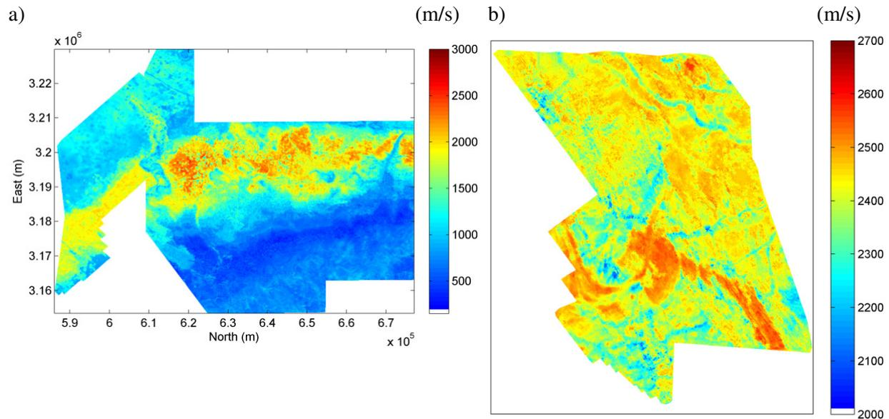
**Figure 1** a) S-wave velocity at 28–35 m of depth (Boiero *et al.*, 2013b); b) P-wave velocity at 40 m of depth below seabed.
