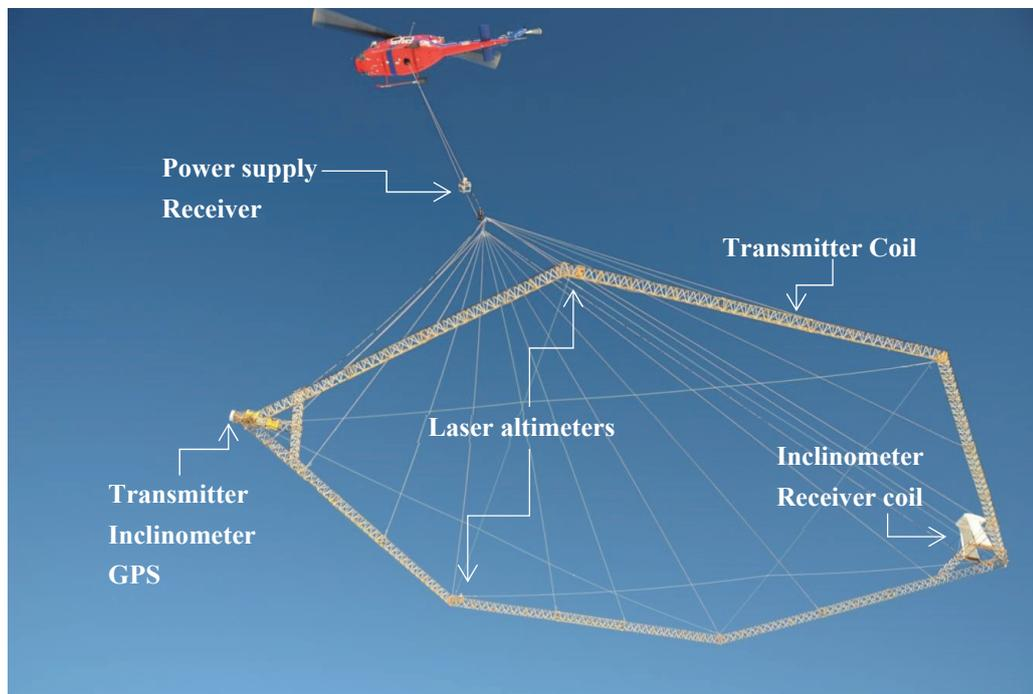
**Figure 1:** The SkyTEM system with indications of the most important devices. The frame in the picture is outdated as the system is now operated with a composite material frame with a smaller air resistance and better stability, but the overall layout is the same.
