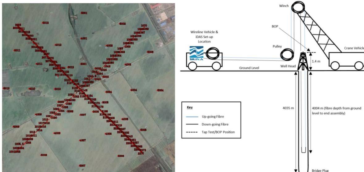
**Figure 1** (Left) Dynamite Shot Position Map the well is located at the centre of the 'X', (Right) Fibre Deployment Schematic.
