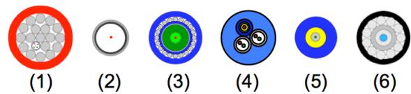
*Schematic cross sections of different optical fiber sensing cables:*
