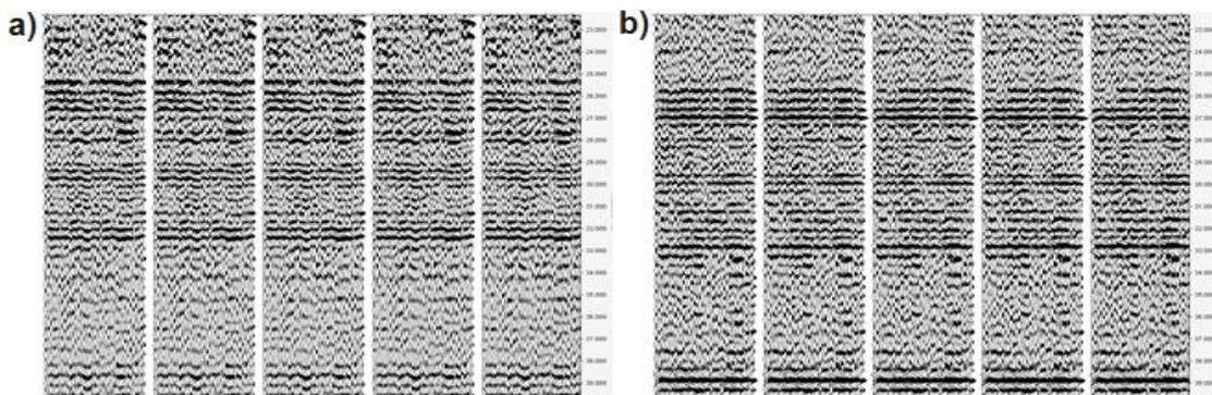
**Figure 1** A group of five neighbouring 3D VSP RTM receiver gathers: a) less accurate model built without any well information, and b) a better model that used bore-hole information in EMB process.
