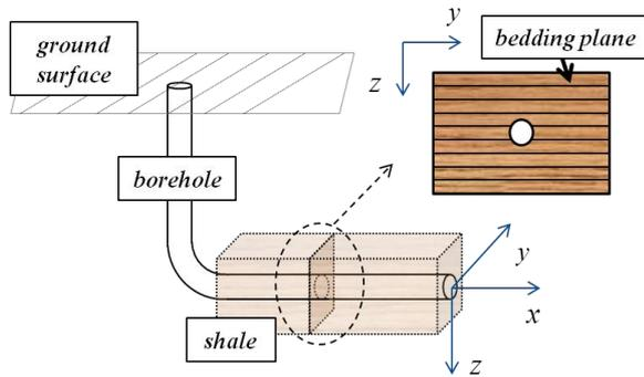
**Figure 6(a)** Hydraulic fracturing in horizontally drilled borehole<sup>(1)</sup>
