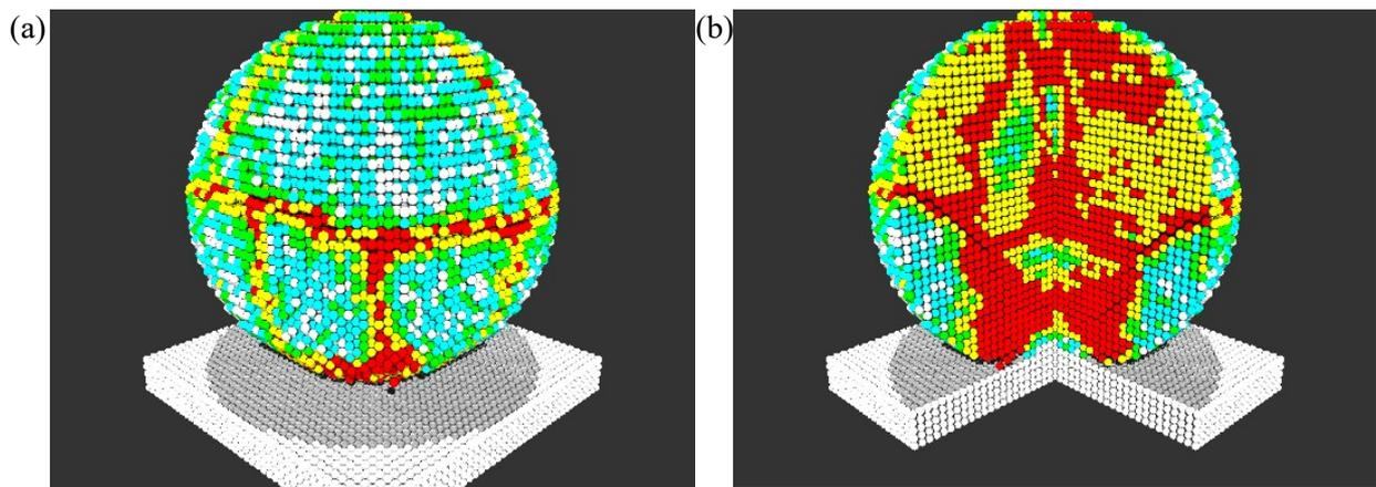
**Figure 3** Macroscopic failure of the brittle sphere. Color of each particle represents the number of broken links. Red: 90 % of links are broken, Yellow: 50 % of links are broken, Green: 30 % of links are broken, Blue: 10 % of links are broken, White: intact part. (a) Overall view and (b) cut a quarter part to visualize inner part of the sphere.
