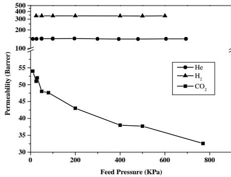
Figure 2. Experimental data on unary permeability of three gases at different permeation pressure
