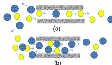
Figure 1 Schematic diagram of two mechanisms: (a) molecular sieving, (b) surface flow.
