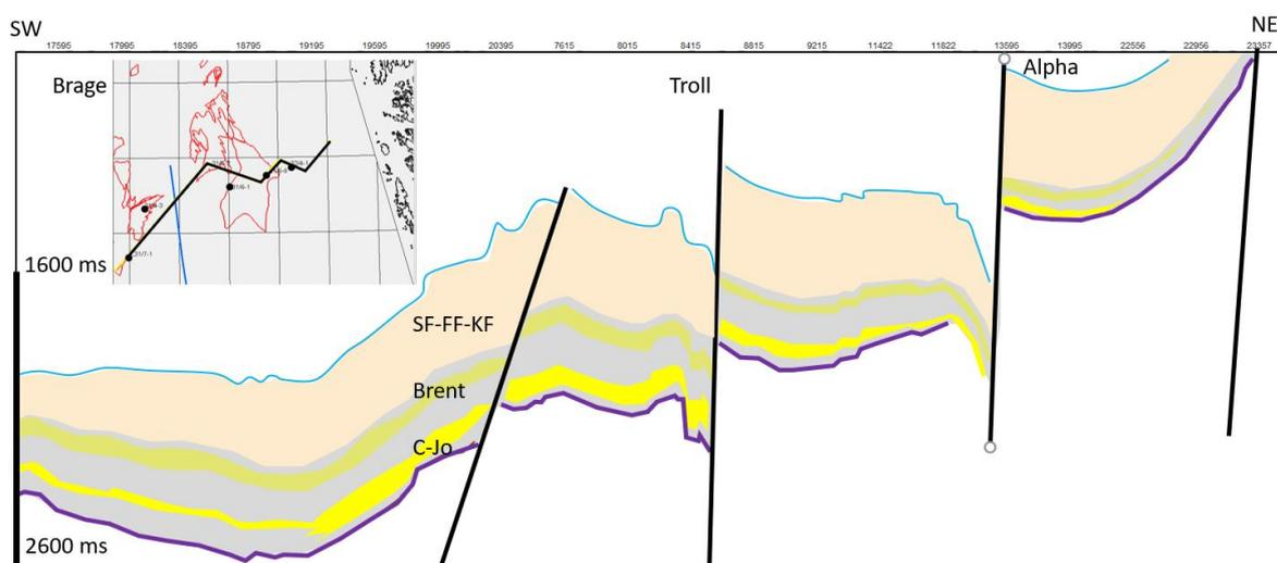
**Figure 3** Interpreted cross-section along seismic composite line. Tied to the wells 31/7-1, 31/4-3, 31/6-1, 31/6-6 and 32/4-1. SF-FF-KF: Heterolithic Sognefjord-Fensfjord-Krossfjord aquifer, Brent aquifer and Cook-Johansen aquifer. Sealing shales are colored light gray. Possible heterolithic aquifer below top Statfjord (purple line).
