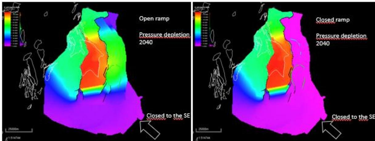
**Figure 6** Simulation results, showing pressure depletion in 2040. Warm colours – large depletion.
