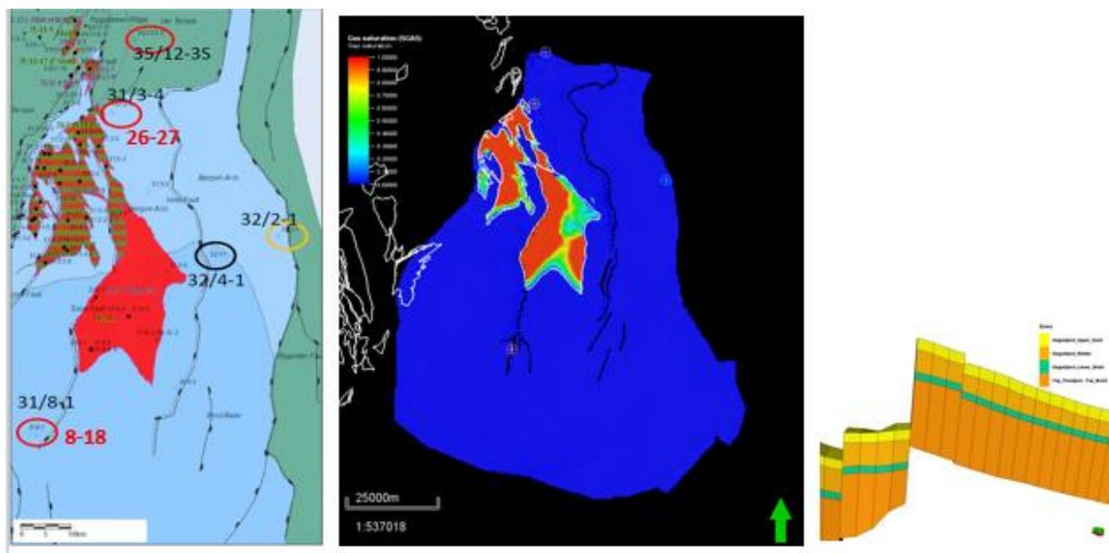
**Figure 4** Troll Field and exploration wells with pressure depletion in bar (red). Data from Fensfjord and Sognefjord Formations.
