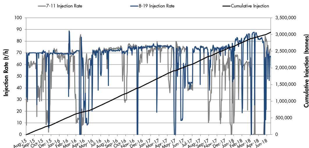
**Figure 1** Quest Injection Totals: Cumulative CO<sub>2</sub> injected into the wells from start-up through to the middle of 2018 (right axis). The blue and grey lines show the average hourly flow rates into the two individual injection wells.
