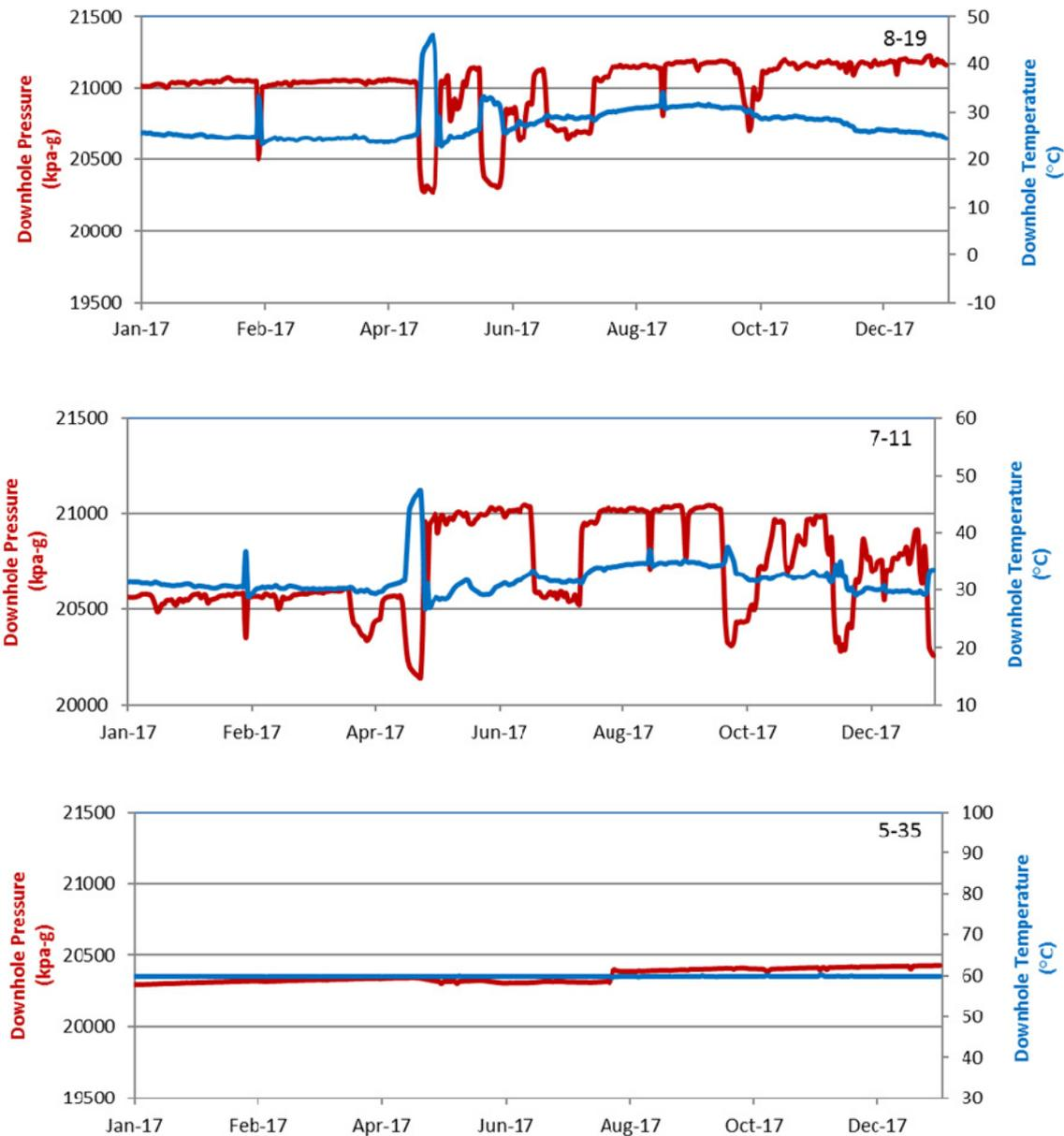
**Figure 2** Quest injection wells downhole pressure and temperature trends from 2017.
