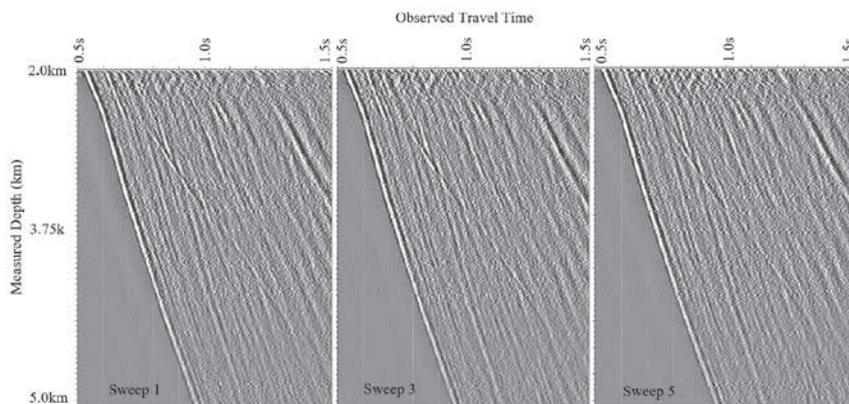
**Figure 10** Raw VSP sweeps using intervention cable in a high deviated well.
