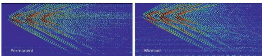
Figure 9 Comparison of the field microseismic event detection on the permanent and wireline engineered fibre.
