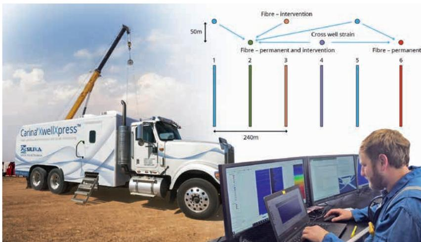
**Figure 4** Multiple well monitoring using permanent and intervention engineered sensing cables. Intervention engineered fibre cable provides a new accessible dimension for crosswell monitoring.
