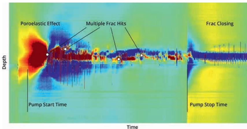
**Figure 5** Colour map of the crosswell strain at depth versus time (600 m-wide over few hours).
