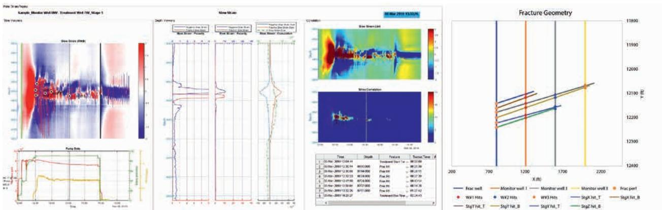
Figure 8 Dashboard of interactive software for strain data processing and identifying the frac hits in real time.
