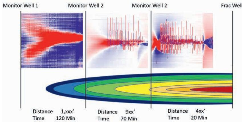
Figure 7 Monitoring the poroelastic effect and frac hits passing through three fibre locations.
