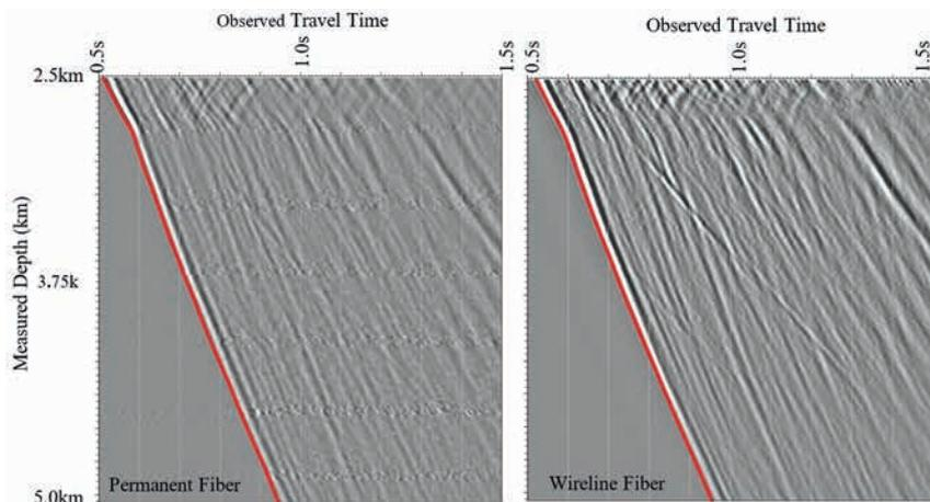
**Figure 11** Permanent installed fibre (left) vs Wireline Intervention cable fibre (right) VSP acquired during the same stage with the same source location.
