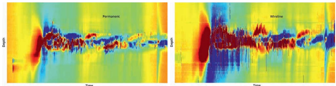
**Figure 6** Low-frequency strain data on the wireline intervention cable (right) compared to the permanently installed cable cemented behind the casing in the same well (300 m-wide over a few hours).
