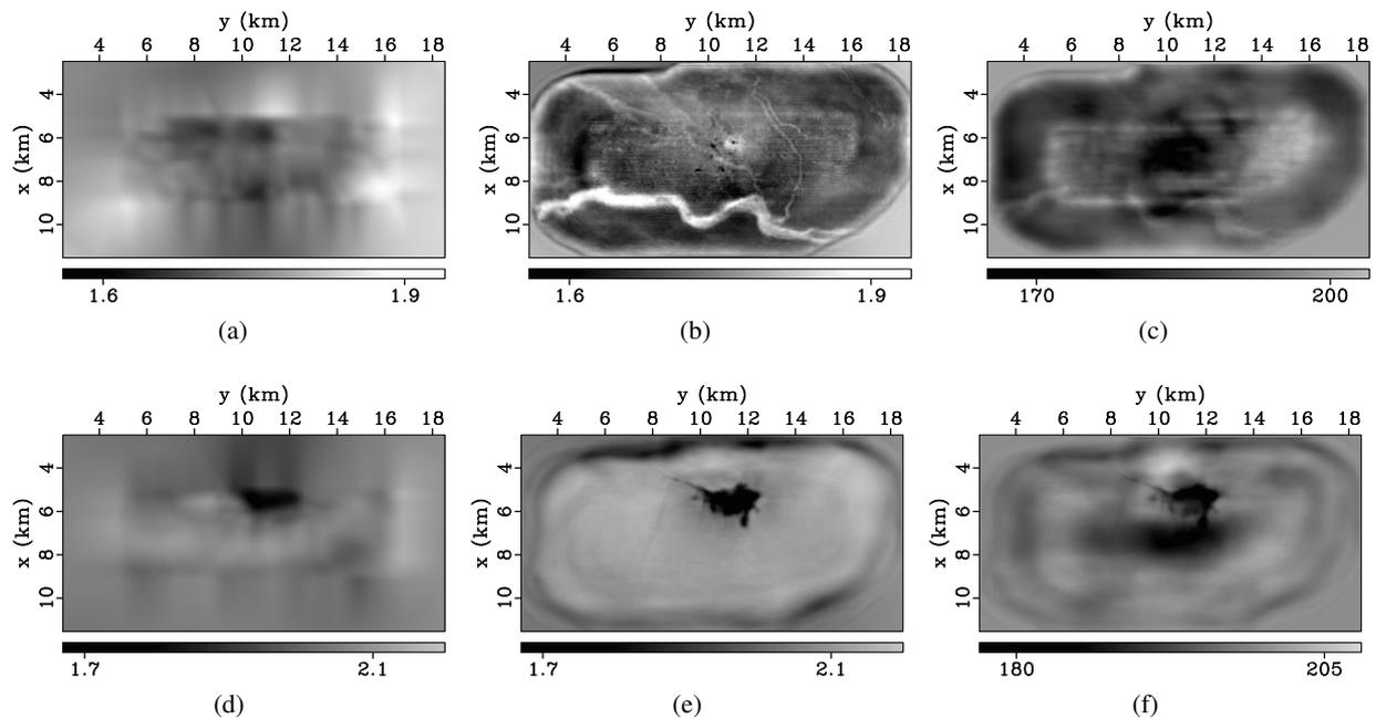
Figure 1: (a) Initial velocity, (b) updated velocity  $V_{p0}$  and (c) updated attenuation  $Q_p$  at depth  $z = 0.2$  km. (d), (e) and (f) are the same at depth 1 km. The units of velocity are km/s.
