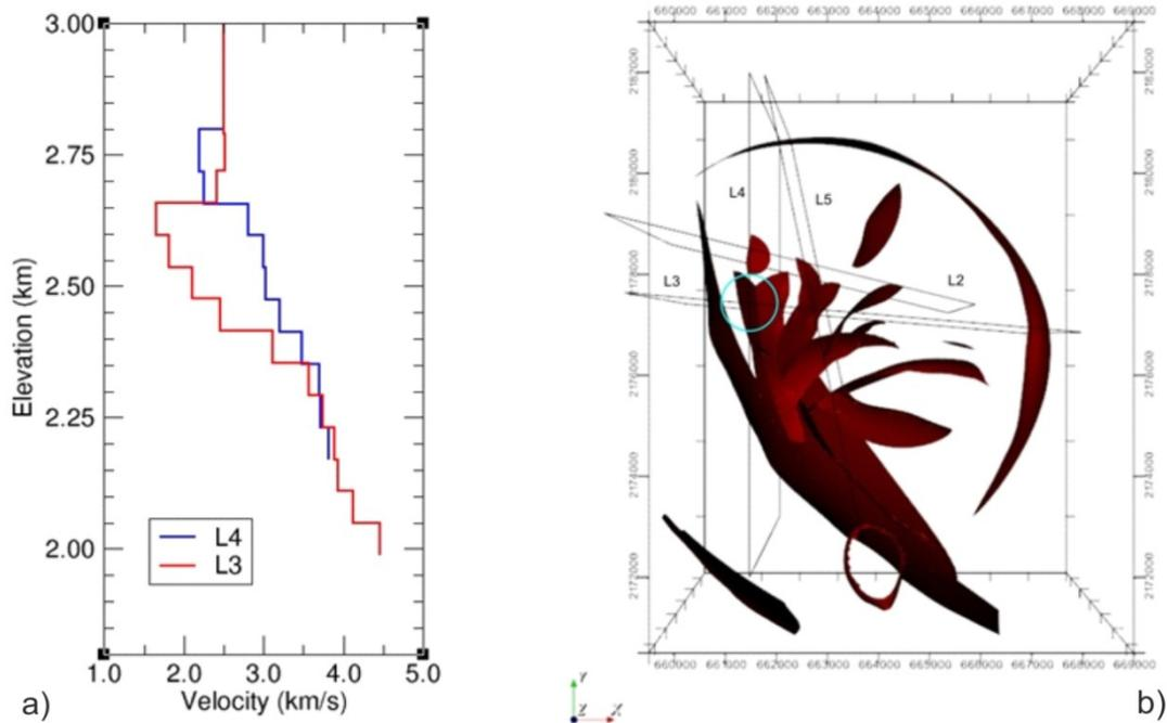
**Figure 3** a) Comparison of P-velocity profiles at the cross between sub-perpendicular L4 and L3 evidences different velocities with possible anisotropy. This zone is characterized by the presence of a shallow fault as shown by the small blue circle in (b) (modified after Calcagno et al., 2018).
