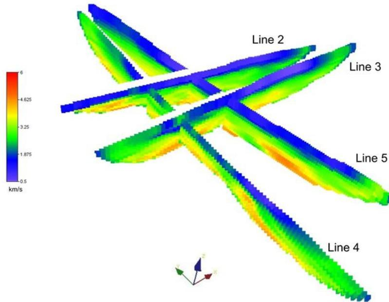
**Figure 1** 3D view of the tomographic inversion for P-velocity of the Los Humeros seismic lines. The velocity is obtained by tomographic inversion of first arrivals picked along the profiles. The maximum depth of investigation is of the order of 500 – 700 m.
