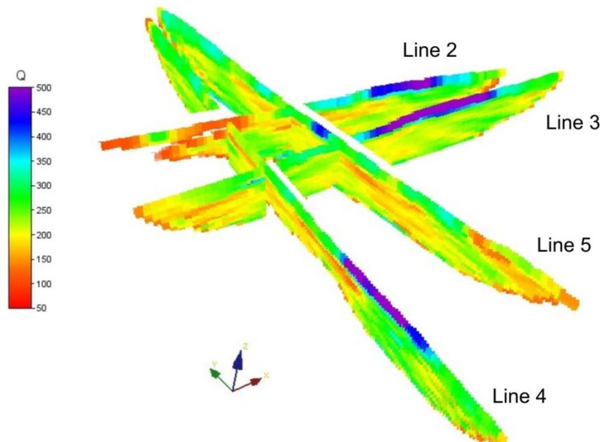
**Figure 2** 3D view of the tomographic inversion for attenuation of the Los Humeros seismic lines.
