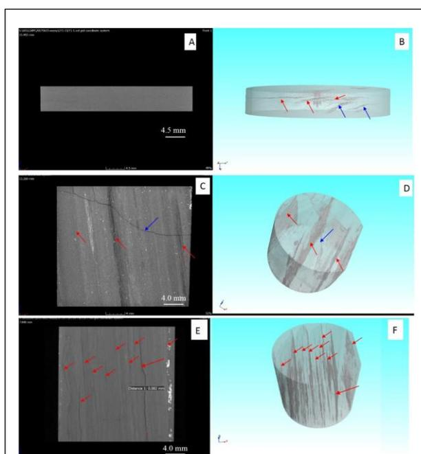
Fig. 1 Micro-CT scans of samples #1 (A, B), #2 (C, D) and #3 (E, F) after solvent flow-through experiments.
