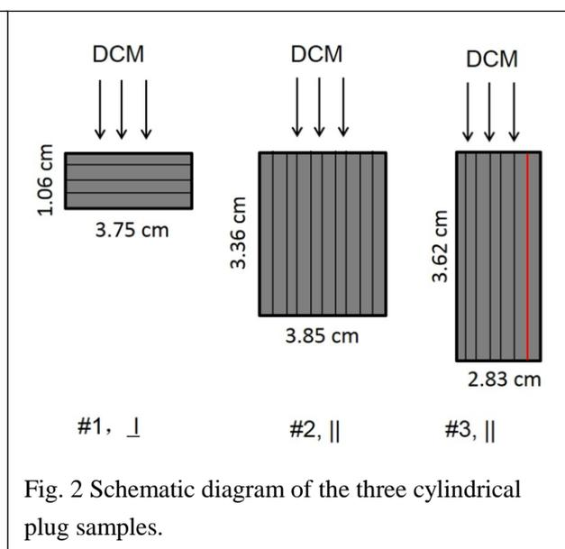
The mobilities of hydrocarbons are controlled by the flow direction and fracture intensity and orientations. For sample #1, DCM flow-through extraction yielded mostly hydrocarbons associated with matrix kerogen. This flow-extracted bitumen was found to be much heavier than that extracted from the other two samples, and to have a lower mobility. The hydrocarbons extracted from the sample #2 were the lightest. For sample #3, containing micro-fractures along the bedding planes, the
