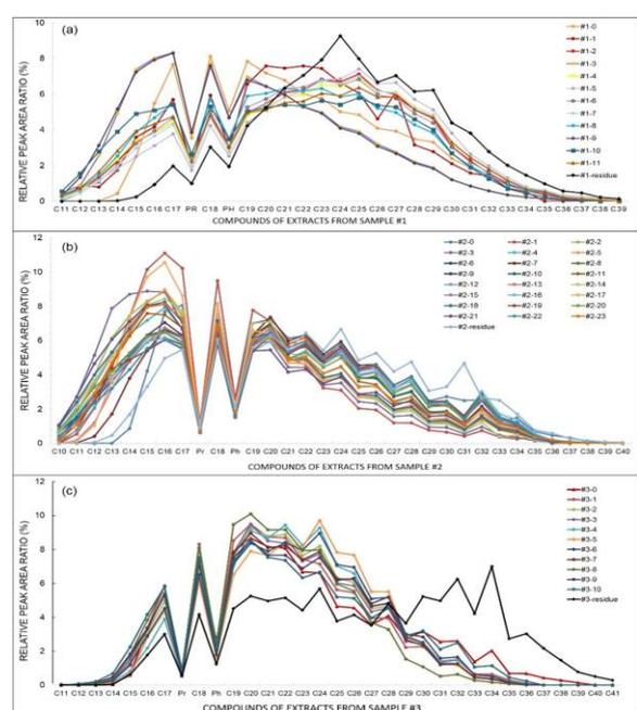
Fig. 2 The relative peak area ratio composition of solvent flow-through extracts of samples #1 (a), #2 (b) and #3 (c).
