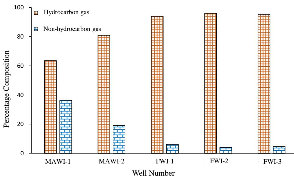
**Figure 1** Hydrocarbon and non-hydrocarbon characteristics of casing gas
