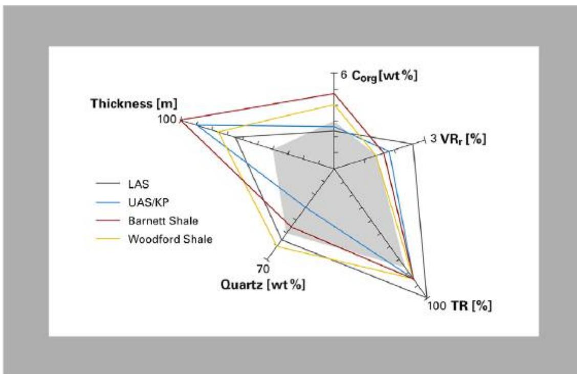
**Figure 1** Comparison of shale gas parameters that control shale gas potential of Mississippian black shale in western Germany with well-known Barnett and Woodford shales (Modified after Jarvie, 2012; Uffmann et al., 2012).
