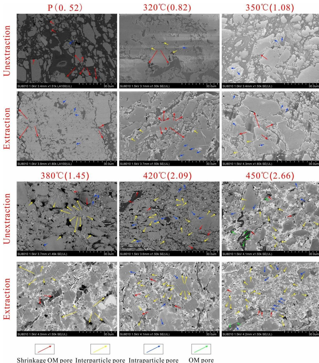
**Figure 1** The SEM images showing the evolution characteristics of pores in shale rocks from the pyrolysis experiments in this work (data in the parentheses showed the values of  $EasyR_o$ ).
