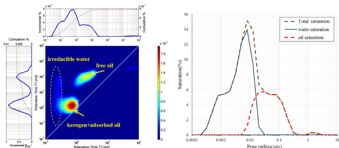
**Figure 1** Representative 2D NMR image and relationships between fluid saturation and pore radius of the Qingshankou first member shale
