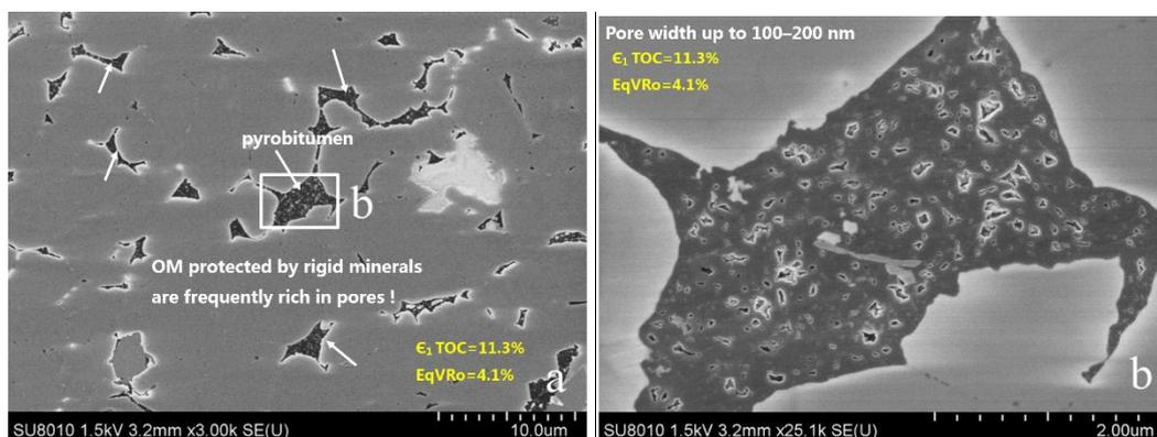
**Figure 1** FE-SEM images of organic pores hosted in pyrobitumen grains of overmature Lower Cambrian shales.
